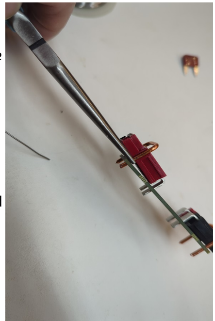
Figure 4: Coaxing staples into PCB
